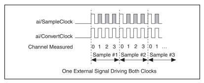
Figure 4-13. Single External Signal Driving ai/SampleClock and ai/ConvertClock Simultaneously
